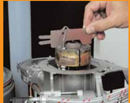
Check the ignition electrodes
