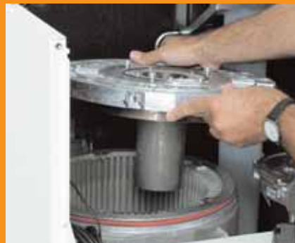
Lift off the lid of the combustion chamber
