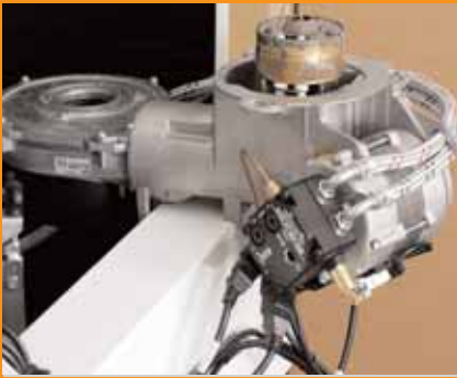
Hook the burner unit into place in the maintenance position
