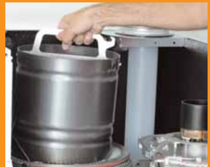
Use the handle to pull out the combustion chamber and spreader unit
