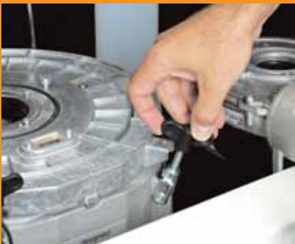
Remove the wing bolts
